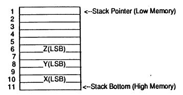
The five empty locations at the top of the Stack are used by the computer to store information about the Stack itself. When using the Stack, however, these positions must always be included in calculating the position of the parameters stored in the Stack.
